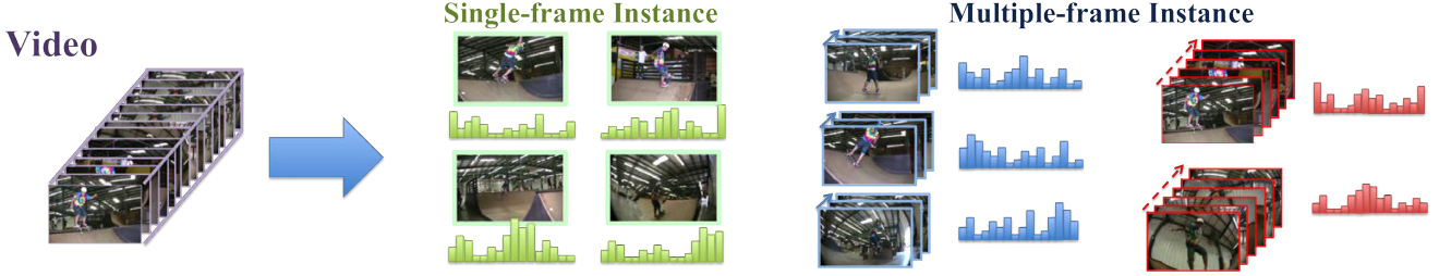
Figure 2. Illustration of multiple-granular instances with different time lengths. In our framework, the instance of minimum granularity is a frame, and instance of maximum granularity is the whole video. Each instance is represented by pooling the included frame-level BoWs.
